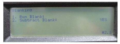
2. Insert and cover your blank (acetone). Press 1 to Run blank.
