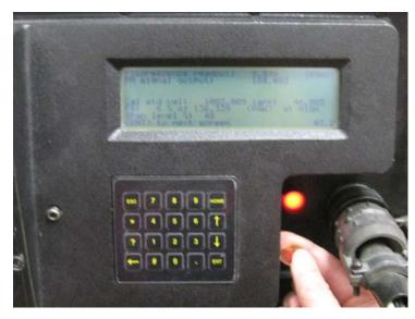
8. When the %FS reaches the designated value, tighten the sensitivity locking screw. For our example this is ≈ 80% of medium
